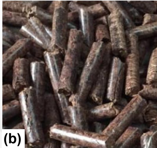
Fig. 1. (a) A creosote straw mixture was produced in this technical route. (b) Pellet fuel produced from a mixture of creosote and straw. (c) Straw directly produced pellet fuel.
