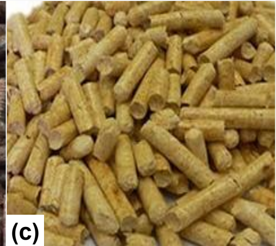
Fig. 1. (a) A creosote straw mixture was produced in this technical route. (b) Pellet fuel produced from a mixture of creosote and straw. (c) Straw directly produced pellet fuel.
