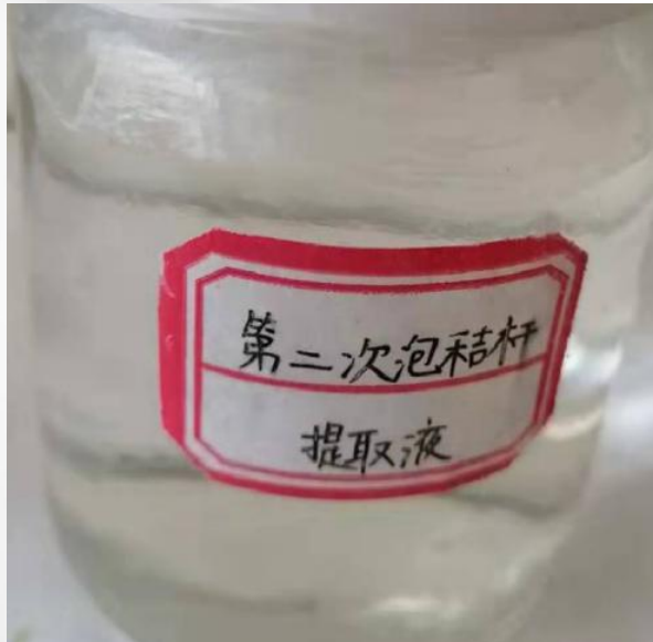
Fig. 2. A refined wood vinegar produced by twice vacuum distillation.
